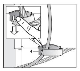
The lower clip (4) can be opened to allow you to take the drain hose out or to feed the mains cable through it.
